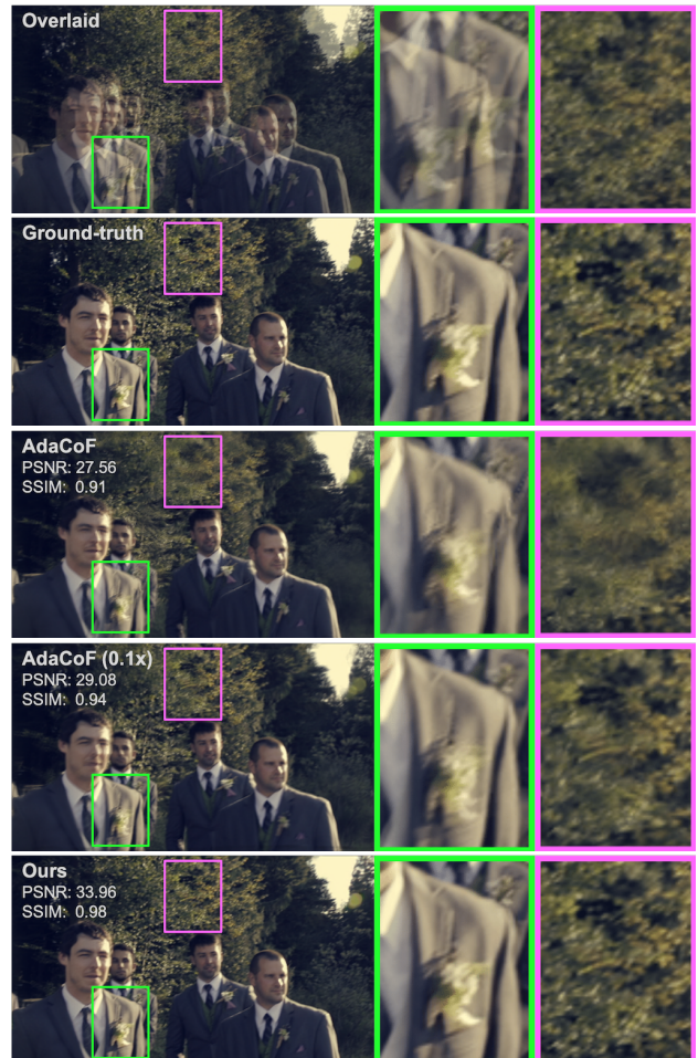
Figure 1. A challenging example consists of large motion, severe occlusion and non-stationary finer details. From top to bottom: the overlaid two inputs, the ground-truth middle frame, the frame generated by AdaCoF [32], the frame generated by the 10× compressed AdaCoF, and the frame generated by our method. The compressed AdaCoF even outperforms the full one in this case.
